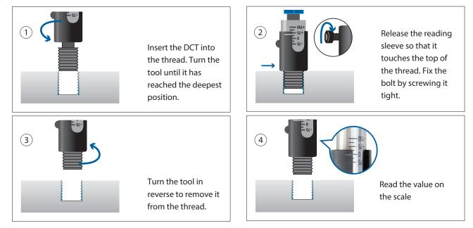
\* The reading value should be used as reference only. To inspect the screw thread please use the limit gauge (refer to p.6).
