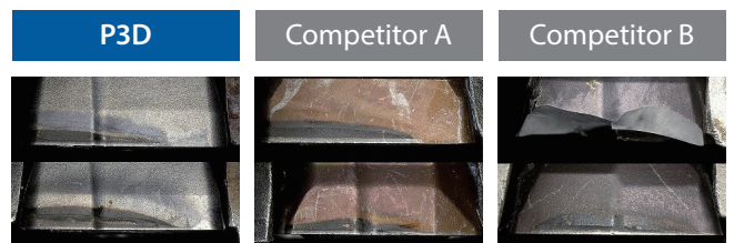
Wear comparison after drilling 48 holes
