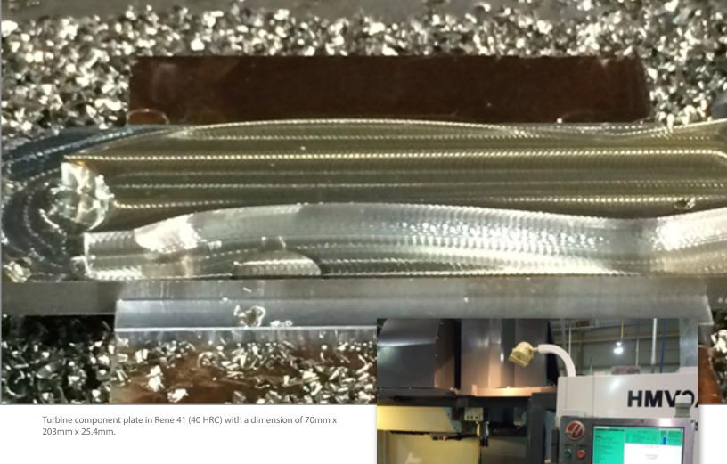
Face milling of the Rene 41 plate in Paradigm Precision's HAAS horizontal machining center using blasomill oil as coolant.
