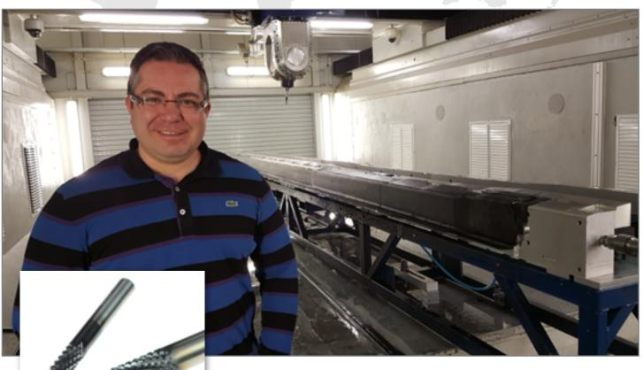
Above: The Z spars are produced in a sophisticated five-axis FOG precision milling machine. TAI's NC Engineering Leader Mr. Onur Bahtiyar oversees the production of the composite wing spars.
